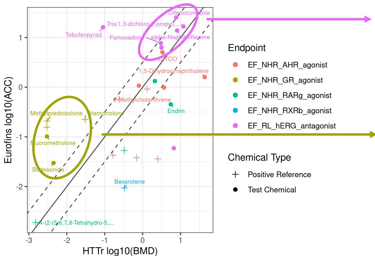
**hERG Inhibitors**: Tier 1 PODs within 0.5-log units of orthogonal endpoint POD or below for 6/9 reference and test chemicals
